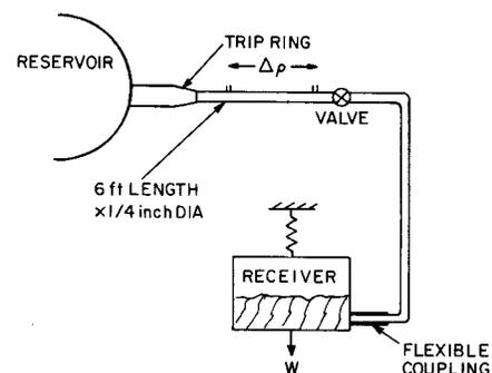
Fig. 1 The apparatus. Pressure difference is created between reservoir and empty receiver. Flow is initiated by opening valve. Pipe pressure drop and receiver weight are continuously monitored.
