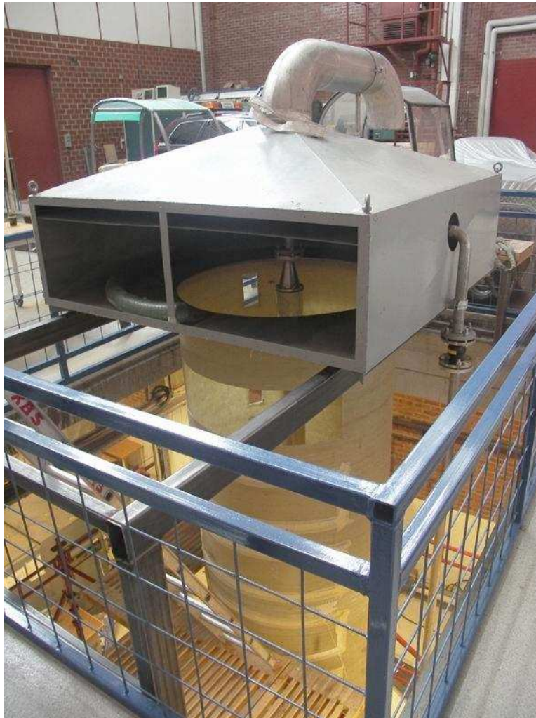
Figure 2.4: Natural convection rig; collection hood.
