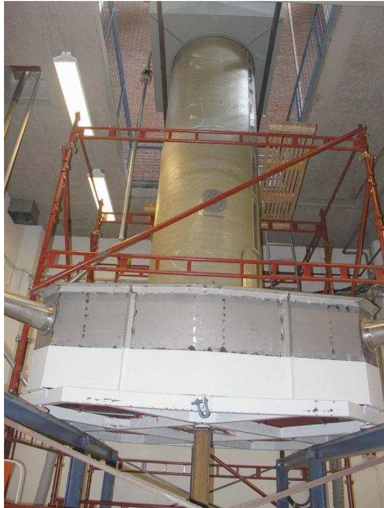
Figure 2.5: Natural convection rig; tunnel and inlet chamber.
